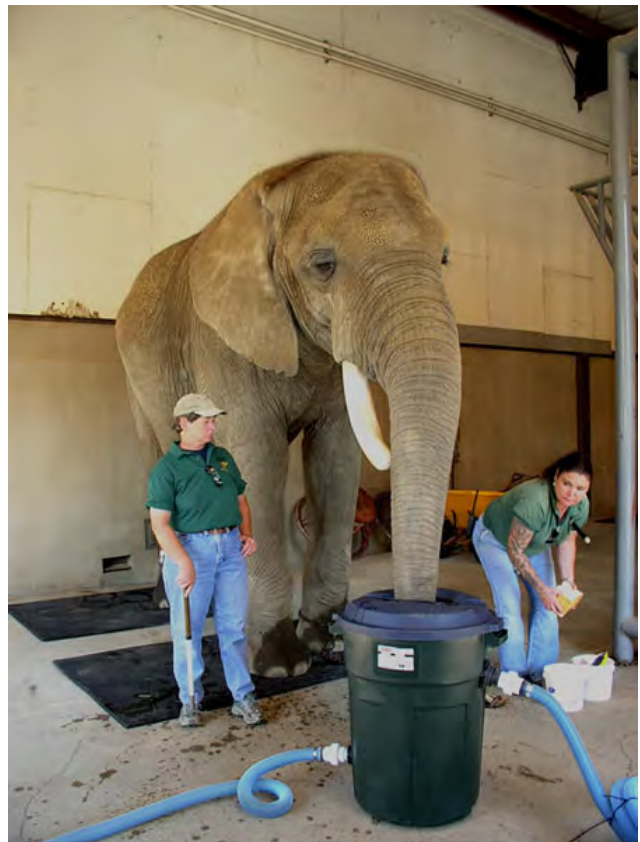
Fig. 3. Flow-through respirometry chamber that was used to measure resting metabolic heat production and respiratory evaporative water loss. Photo credit: T. M. Williams.
